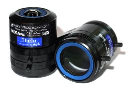
Theia's newest megapixel offering, the SL940A telephoto lens, provides full 5 megapixel resolution to zoom in and deliver high detail images. The IR-corrected, CS mount lens has a focal length of 9 to 40 mm, and is designed to let the user take full advantage of the  $\frac{1}{2}.5$ " sensor used by Dallmeier's new camera. And at a compact 50mm long, it easily fits in the dome profile.
